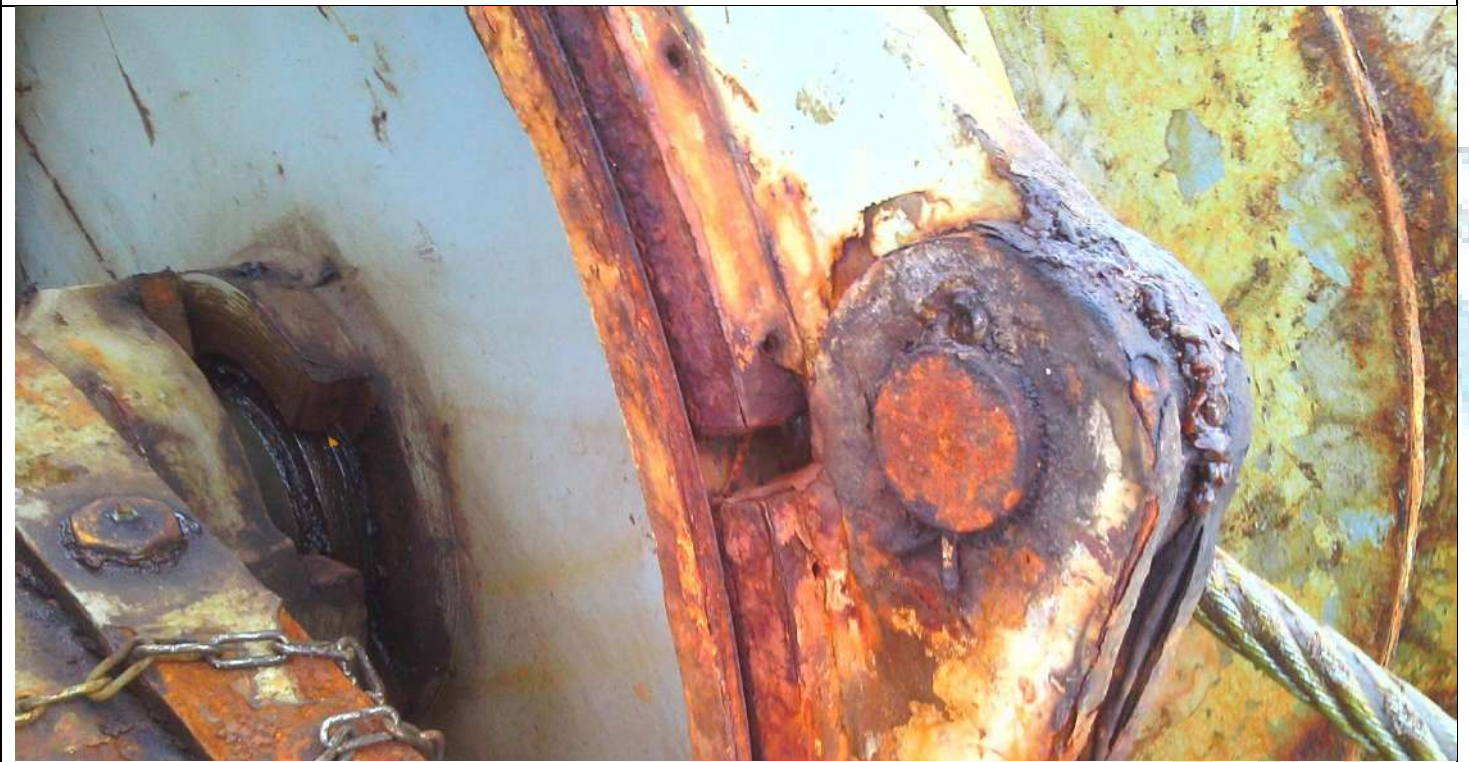
ANY MAJOR DEFECT – WINCH CORROSION
