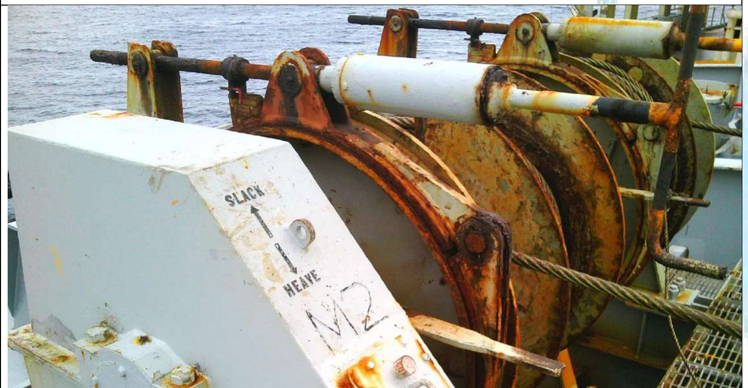
ANY MAJOR DEFECT – WINCH CORROSION
